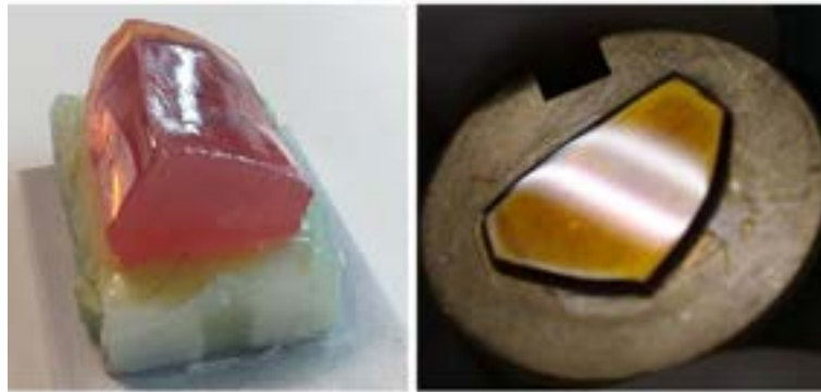
Figure IV.5. Images of the bulk YSZ-Ce sample uncut and unpolished (left) and after cut and polished with the 3 and 1 \mu\text{m} diamond suspensions in water and cloth.
