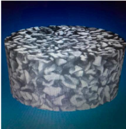
Fig. 5: Micro-CT images of the structure of the particulate graft with a resolution of 11.8 pixels, a scanning time of 3 hours and an exposure time of 8500 ms.
