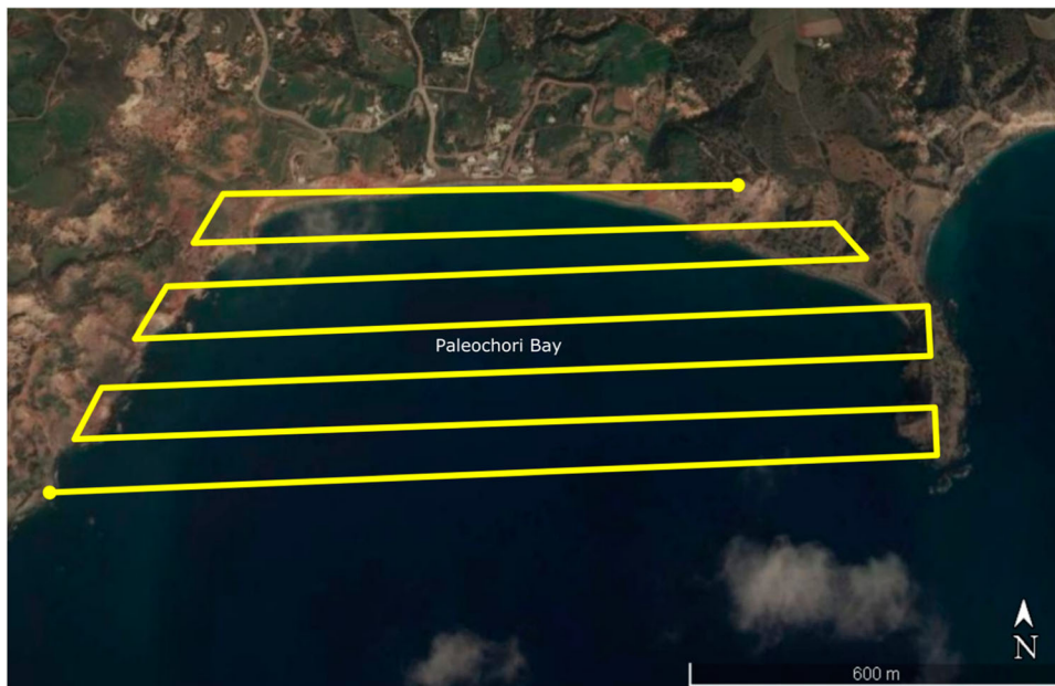
Figure 4. Flight plan for the UAS survey. The flight plan was calculated using the MapPilot software.
