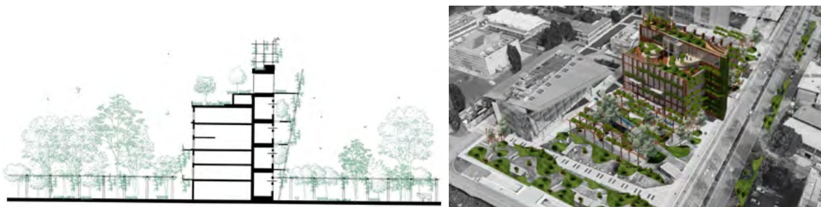
Figure 34. Section and impression of the building, showing the double skin façade addition and the introduction of natural elements.
