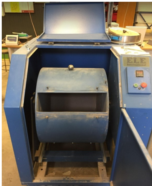
Figure 4.6: Los Angeles test machine for testing resistance to fragmentation
