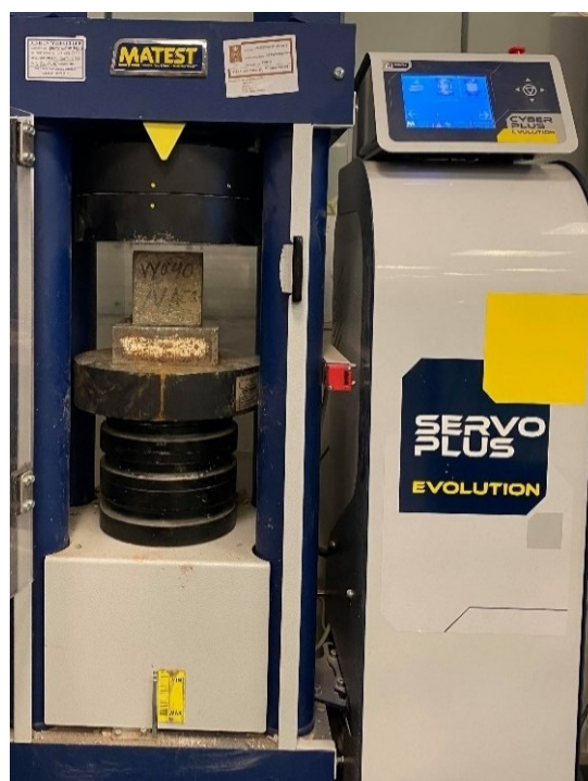
Figure 4.14: Compression testing machine used for testing compressive strength of concrete
