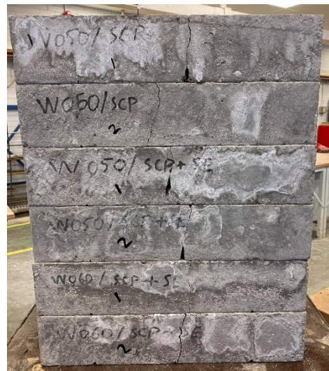
Figure 5.25: Flexural failure mode of some of the RAC beams
