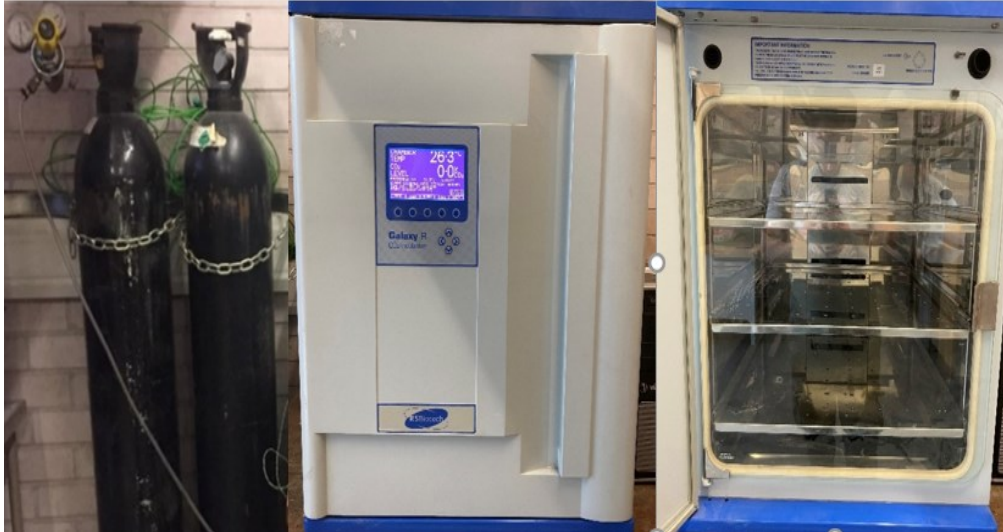
Figure 3: CO 2 incubator used for the CO 2 treatment of recycled aggregates
