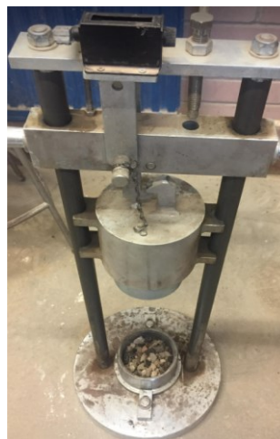
Figure 4.5: Aggregate Impact Value (AIV) test apparatus
