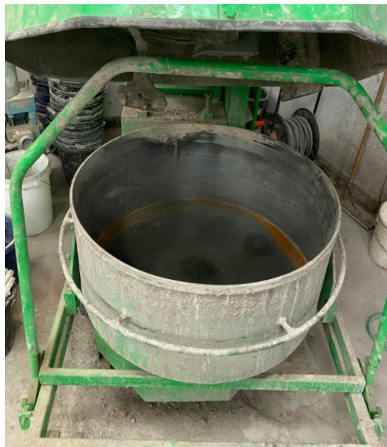
Figure 4.10: Croker Cumflow RP100 XD MK2 rotating pan mixer
