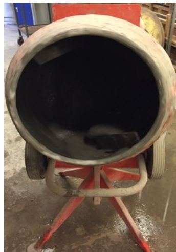
Figure 4.7: Conventional concrete mixer machine for recycled aggregates water washing treatment
