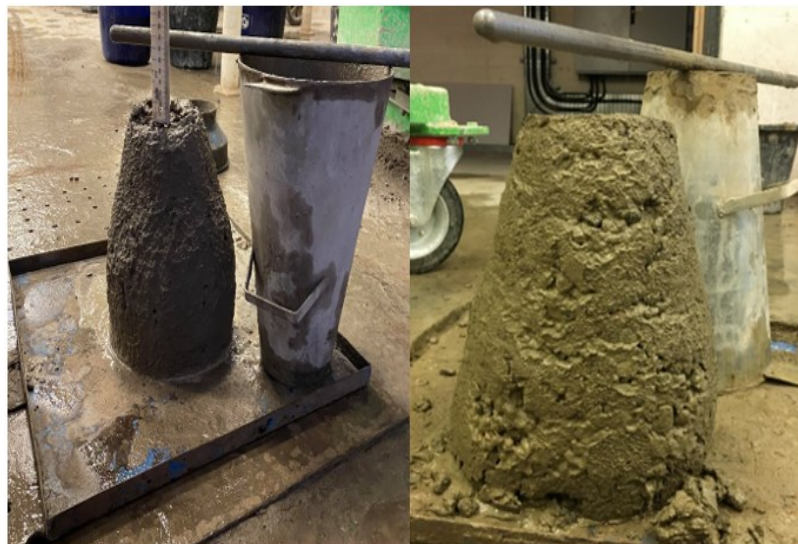
Figure 5.18: Slump test for some of the concrete mixes
