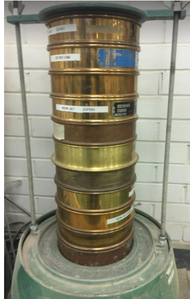
Figure 4.2: Sieve shaker device for determination of particle size distribution
