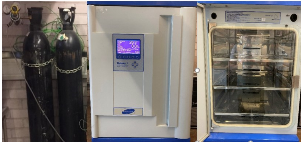
Figure 4.9: CO 2 incubator used for the CO 2 treatment of recycled aggregates
