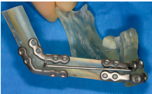
Fig. 1. Stereolithographic model of the planned Brown type IIc hemimandibulectomy defect reconstructed with a two-segment fibular free-flap and fixation using a printed titanium alloy miniplating device with detachable patient-specific plate positioning jig.
