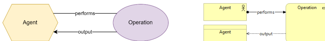
Figure 13. Translation of a KAOS agent (left) to both an ArchiMate business actor and business object (right)
