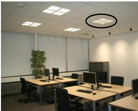
Fig.1: Experiment room - luminaire above desk 4 (black circle), which was dimmed during the experiment. Screens were closed to exclude daylight.
