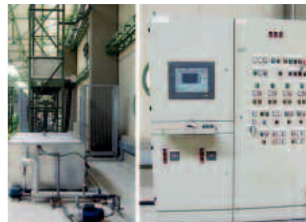
Figure 6 - Buoyant jet thermal-hydraulic system with the process computer
