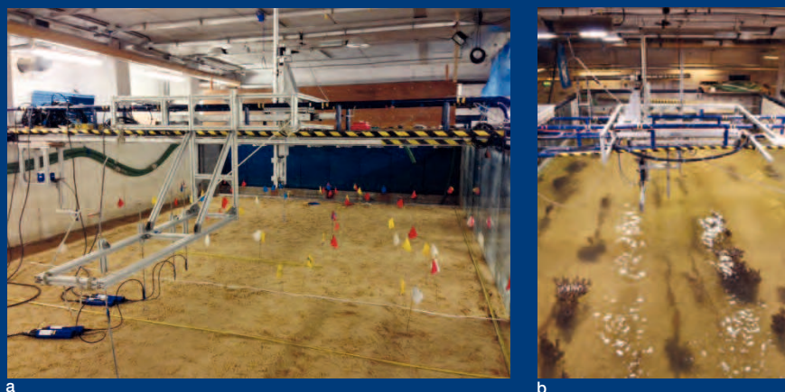
Figure 2 - (a) Experimental set-up in the Total Environment Simulator, University of Hull with flags showing the locations of macroalgae to replicate field distribution. (b) View looking downstream in flume during experiments
