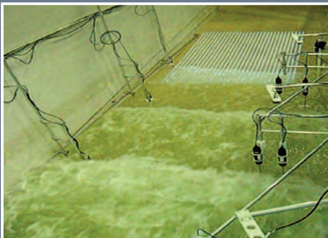
Figure 1 - Illustration of the newly developed grid of optic points for the swash zone (a, left panel) and the bed form and suspended load acoustic imager for the nearshore zone (b, right panel)
