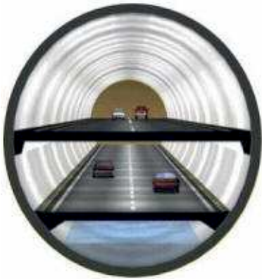
Figure 1. Typical Tunnel Cross-Section at Traffic Compartment
