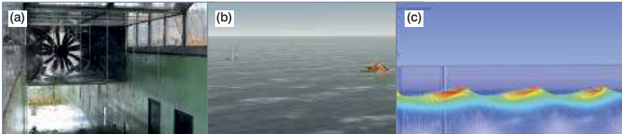
Figure 4. (a) Large wave and wind flume, (b) real time maneuvering simulation for transportation of a wind turbine foundation and (c) CFD model for wave forces on a wind turbine
