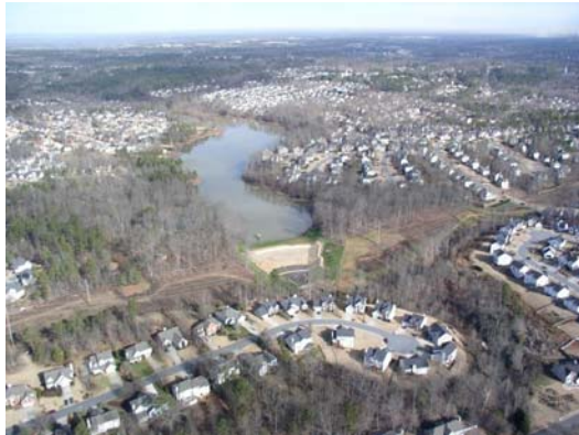
Figure 1 A high risk dam in Georgia, USA, due to significant urban development at the downstream (NRCS, 2008).
