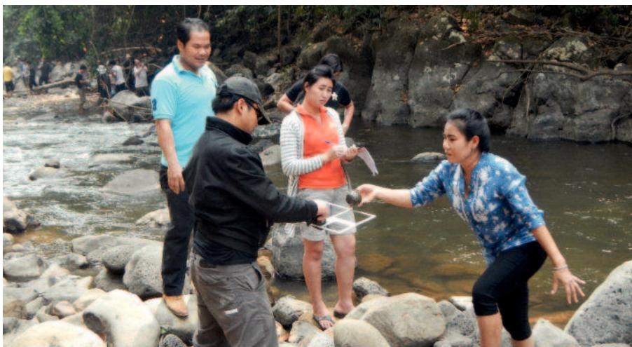
Figure 3. Mr. Vithounlabandid THOUMMABOUT leads a team of MEM-DEPP engineers learning to estimate bed material size with a gravelometer (March 2015)
