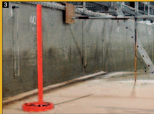
Figure 3 - Wave gauges, suction bucket pile and Vectrino (on right) prior to a scour test
