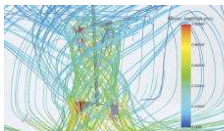
Figure 8. Streamlines across mixers simulated with rotating reference frames
