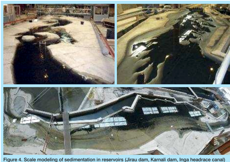
Figure 4. Scale modeling of sedimentation in reservoirs (Jirau dam, Karnali dam, Inga headrace canal)
