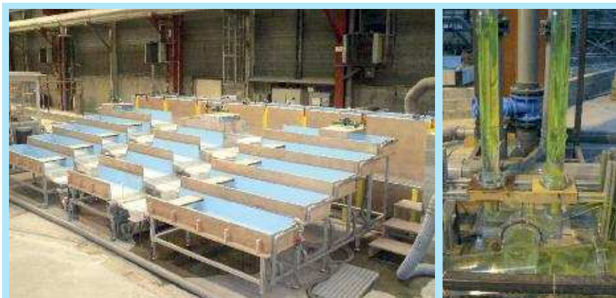
Figure 3. Scale model of a 30 m lift lock with 5 saving basins and of hydropower scheme surge shafts
