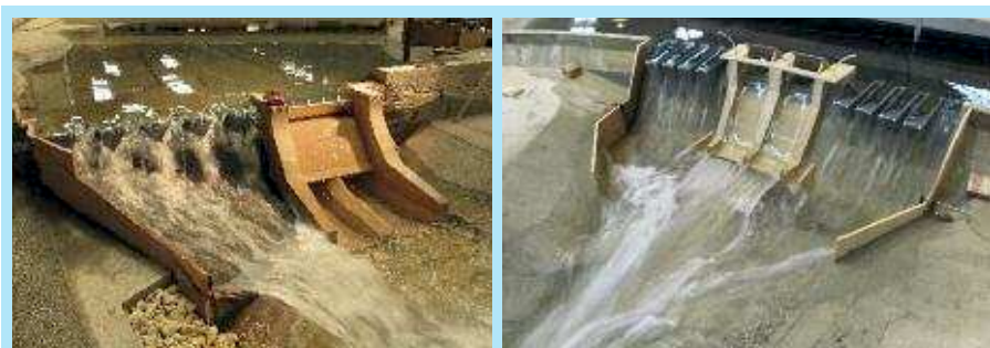
Figure 2. Scale modeling of dam rehabilitation projects with upgrading of flood spillways
