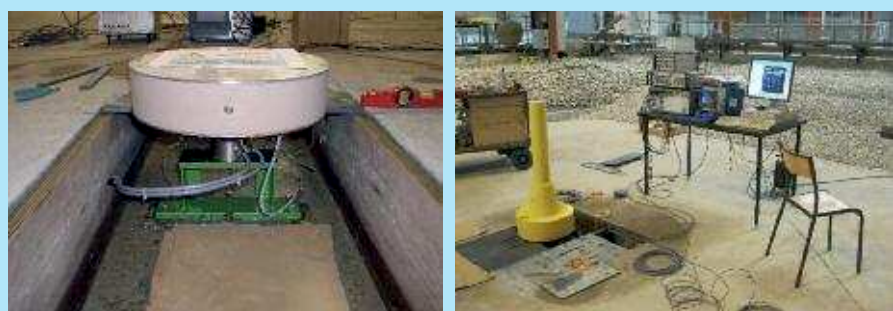
Figure 7. 6-components strain gauge balance for measuring wave loads on a gravity-based structure (GBS) concept for offshore wind turbine development
