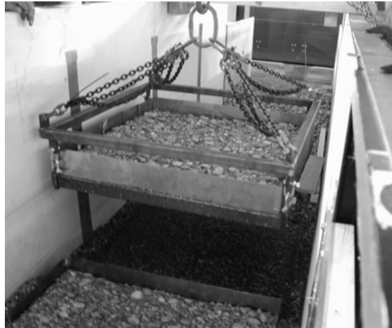
Figure 1 The equipment used to rotate the water worked bed by 90° to form bed 2.
