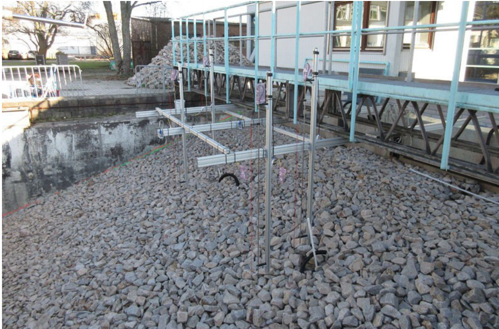
Figure 11: Wave basin with the model of the embankment and some sensors.
