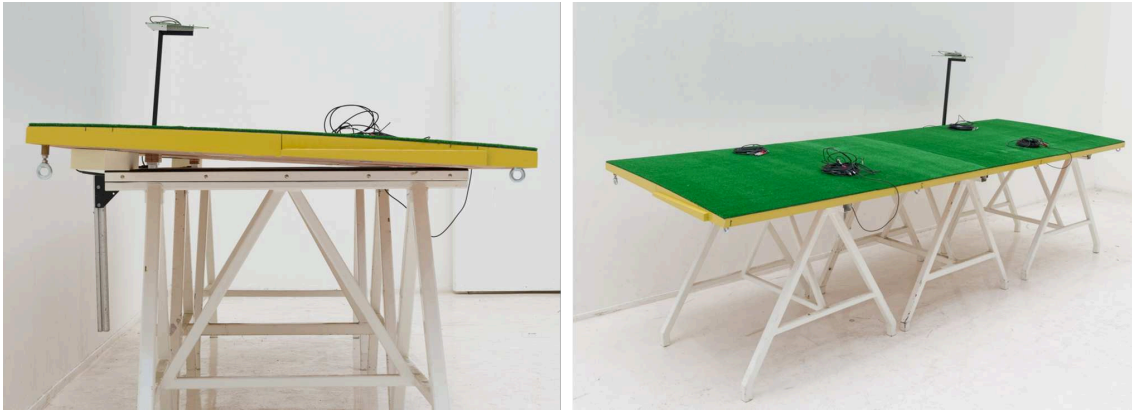
Figure 2: Photos of as-built model with grass cover, including instrumentation, in the same orientation as during the basin tests.
