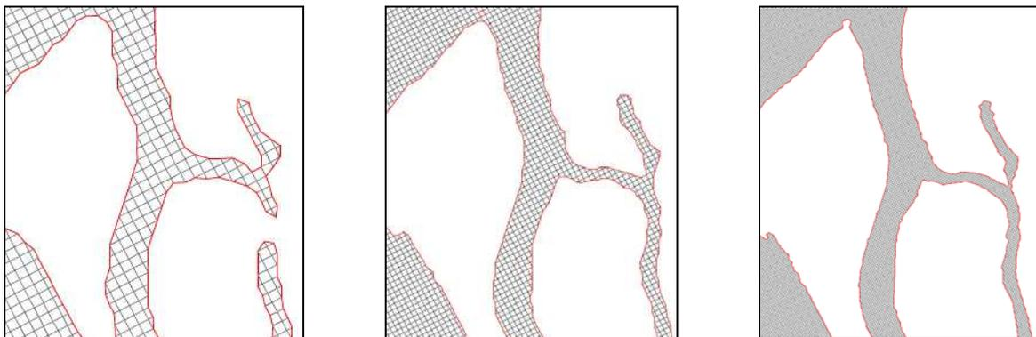
Figure 4 Spatial structure of the grid for a grid resolution of 50 m, 25 m and 10 m and a water level of 101.37 m ASL. The position of the depicted area is shown in frame A in Figure 2.
