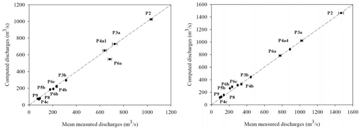
Figure 6 Computed versus measured discharges for the flow situation from 24<sup>th</sup>/25<sup>th</sup> (30<sup>th</sup>) June 1997 (left) and 9<sup>th</sup>/10<sup>th</sup> July 1997 (right), computed with a grid resolution of 10 m.
