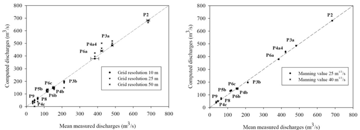
Figure 5 Computed versus measured discharges for the flow situation from October 21<sup>st</sup> to 23<sup>rd</sup> 1996, for different grid resolutions (left) and Manning values (right).
