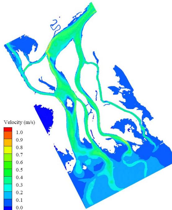
Figure 8 Computed flow velocities on the water surface for the flow situation of 21<sup>st</sup> to 23<sup>rd</sup> October 1996, Lake stage 101.37 m ASL, Discharge  $712 \text{ m}^3/\text{s}$ .
