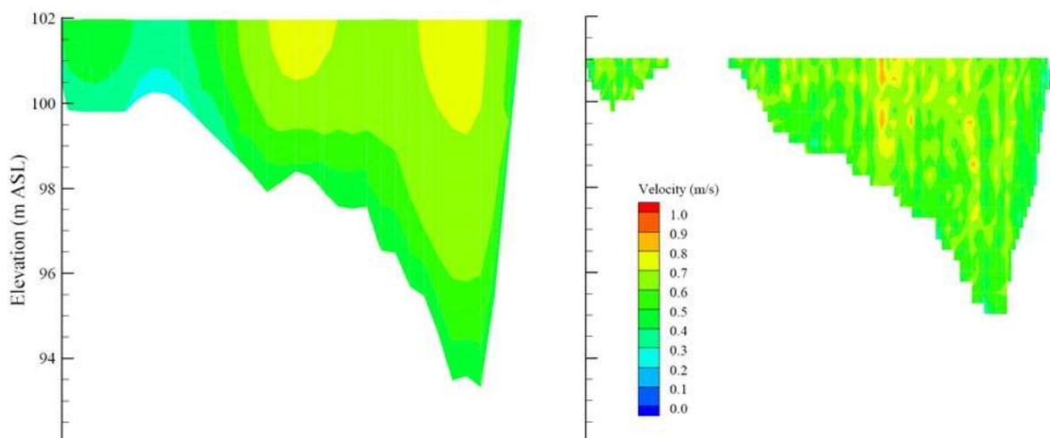
Figure 7 Flow velocities at cross-section P6a for the flow situation on 9<sup>th</sup>/10<sup>th</sup> July 1997, left computed with SSIIM, right for one of four ADCP measurements of the profile.
