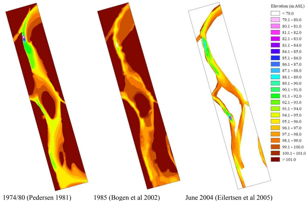
Figure 3 Bed levels of the Storråka channel at different times (See frame B in Figure 3).
