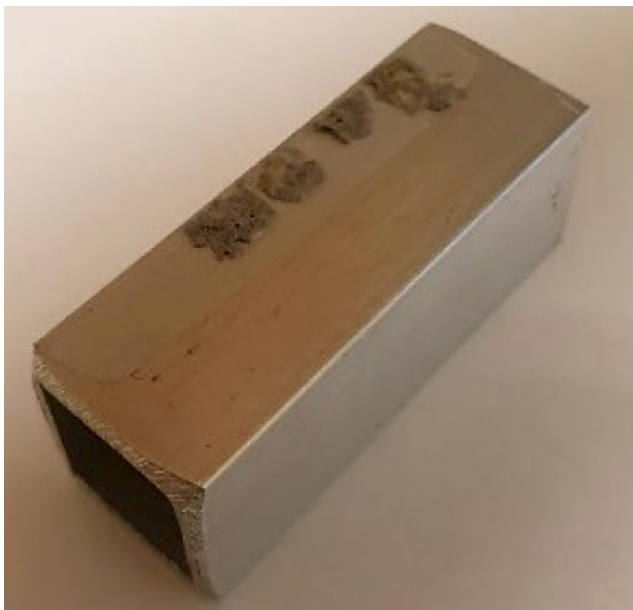
Figure 9 –Top: Scaled material after sieving. Bottom, left: Flakes mounted on a hollow steel bar with quadratric cross section by double-sided tape. Bottom, right: Digital photos taken perpendicular and parallel to the surface of the steel bar made it possible to determine thickness ( T ), length ( L ) and width ( W ) of the individual flakes accurately. (Illustrations from [14]).
