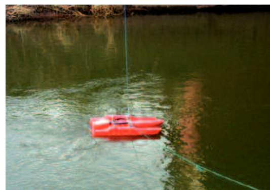
Figure 1 – ADCP gauging on the River Teme, England.
