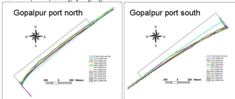
Fig. 3. Shoreline change (berm position) along Gopalpur port north and south
