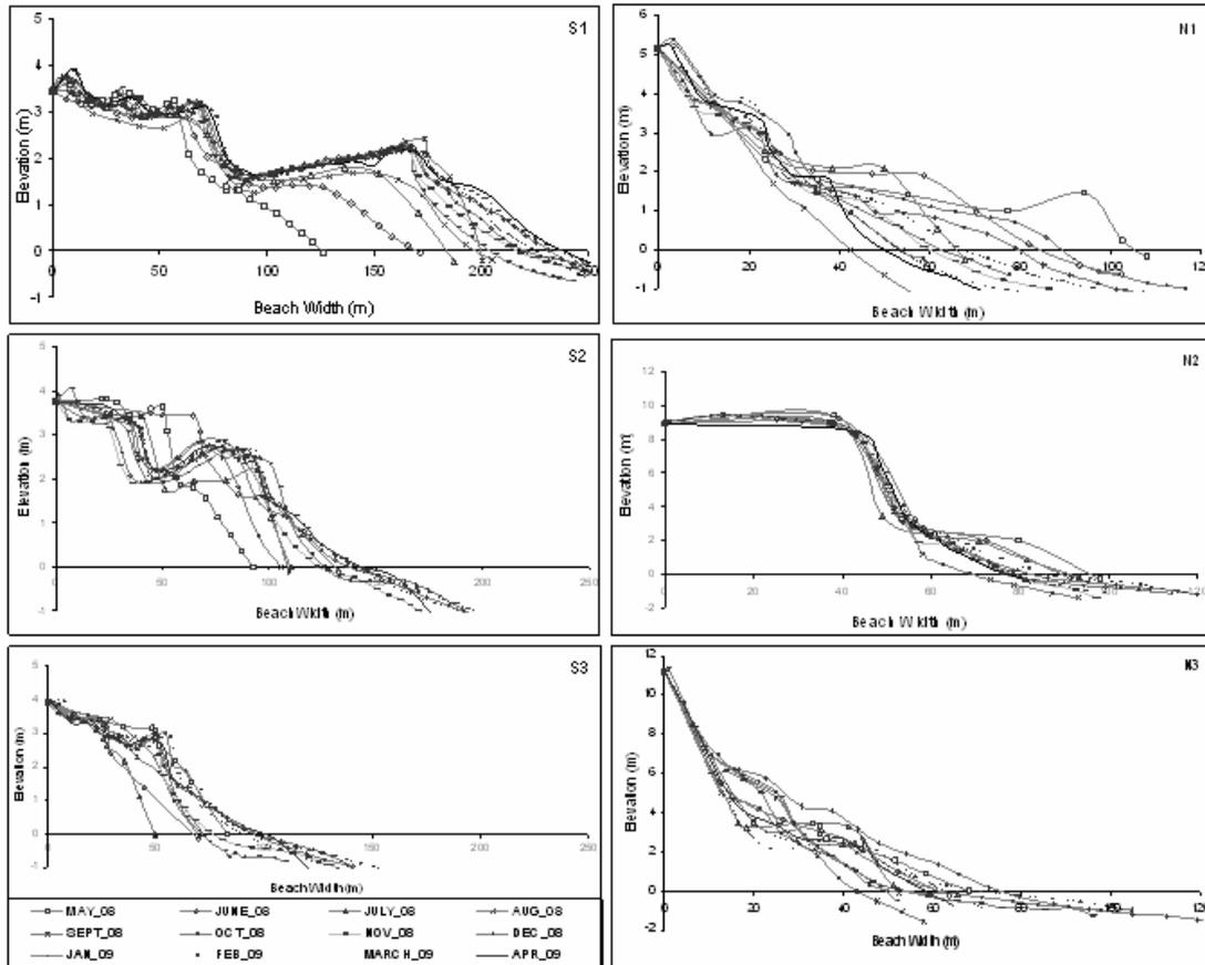
Fig. 2. Beach profile near Gopalpur port; south of south groin (S1, S2, S3) and north of north groin (N1,N2,N3).
