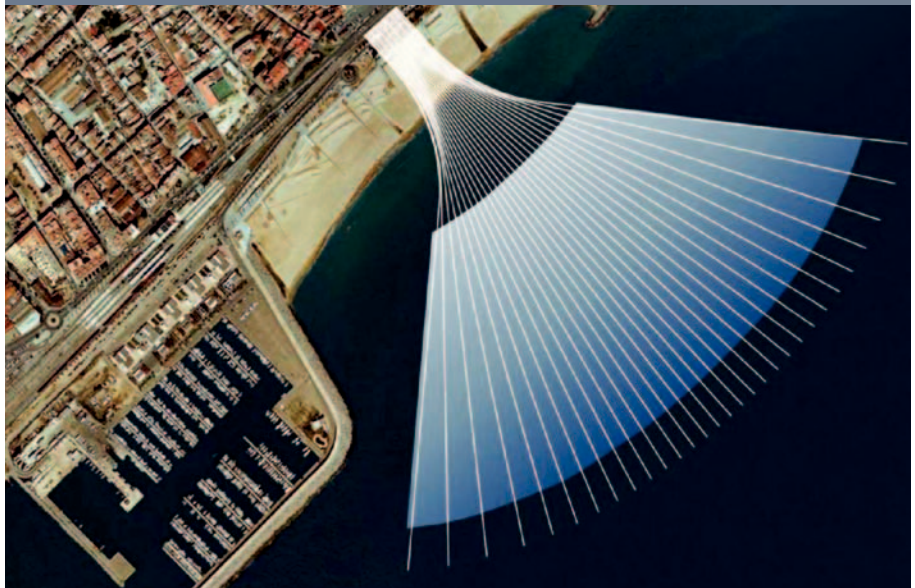
Fig. 3: Seawater Desalination intake system at Barcelona (Spain). Several horizontal subseabed drills with filtration region shown in light blue provide large flows of high quality seawater due to the pre-filtration within the seabed (Courtesy: Neodren system).
