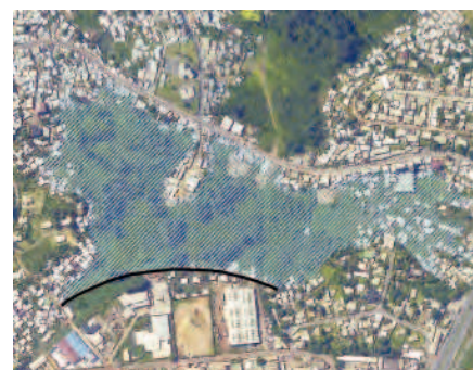
Figure 8 - Example of temporary floodwater storage area
