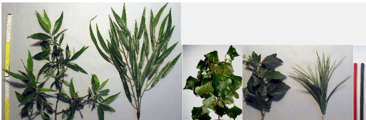
Figure 4 Side elevation of the investigated vegetation elements (from left to right: natural willow; artificial willow; natural poplar; artificial poplar; artificial sedge; plastic cylinder; and steel cylinder; each colour mark on the scale is 10 cm)
