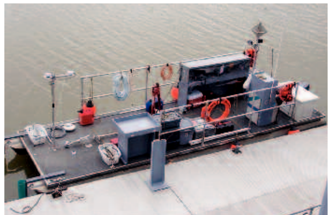
Figure 4 - One of Alden's boats for field measurement equipped with DGPS navigation, bathymetry and velocity measurement equipment
