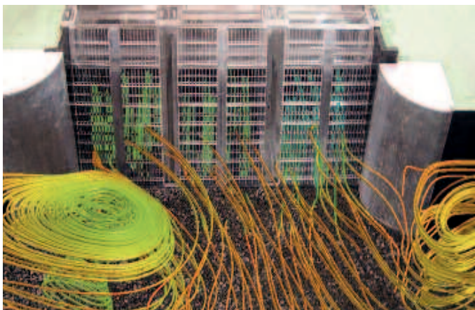
Figure 3 - Computational Fluid Dynamics (CFD) model results superimposed on a physical model for a combined CFD – physical model study
