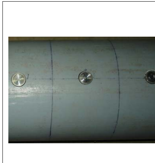
Fig. 2. Intake pipe housed with pressure sensors
