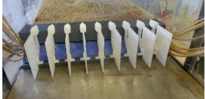
Figure 2. Overall view of MiCas system from downstream with membrane boxes installed in the flume visible in blue. Each membrane box constitutes a bin
