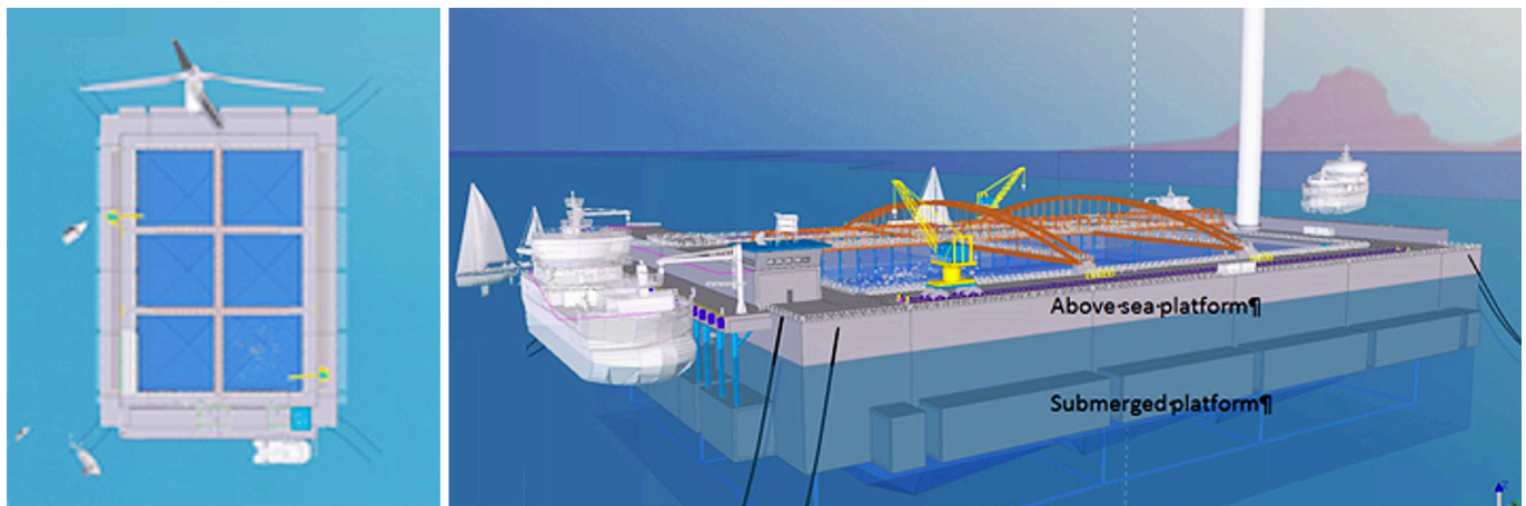
Figure 1 | The Design of the full-scale multi-purpose offshore platform 'The Blue Growth Farm'.
