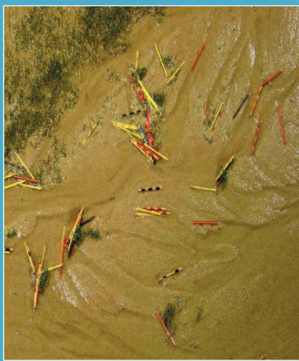
Figure 3 - Pieces of large wood stranded on a bar next to a big island in the flume (on the left) and on the Tagliamento River, in Italy (on the right). Flow is from left to right
