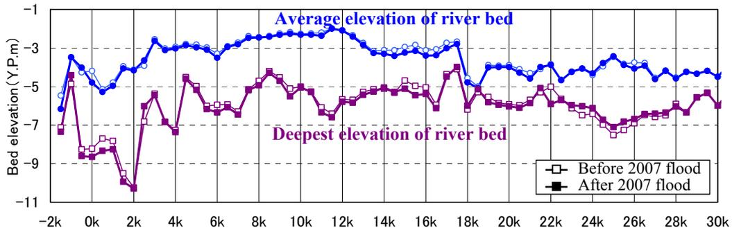
**Figure6. Bed elevation change before and after 2007 flood**
