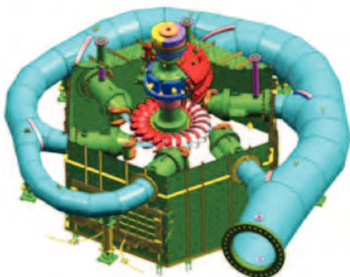
Figure 1 - Left: global view of a Pelton unit. Right: flow simulation in a 6-jets Pelton runner with ASPHODEL. Computational particles colored by their velocity in the absolute frame of reference. Blue means low and red means high velocity magnitude values
