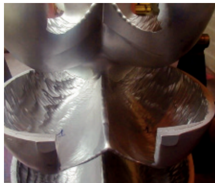
Figure 5. Abrasion on Pelton runner (source: EDF)
