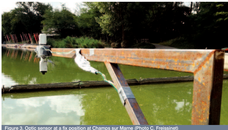
Figure 3. Optic sensor at a fix position at Champs sur Marne (Photo C. Freissinet)
