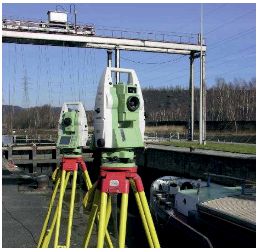
Figure 1. Measuring vessel position at Roselies lock
