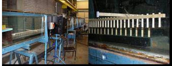
Figure 2 Experimental compound channel.
