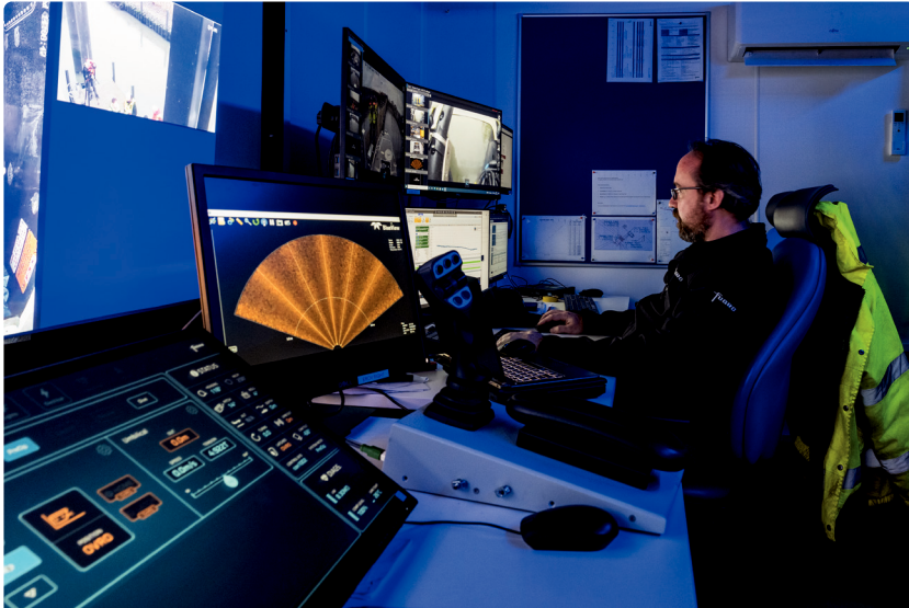
Fig. 4: Operational control of the USV is done from dedicated or mobile remote operations centres as well as quality monitoring of the acquired data
