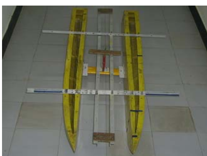
Fig. 7. Catamaran model with straight foil
