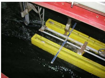
Fig. 13. Flow pattern around the catamaran model with dihedral foil
