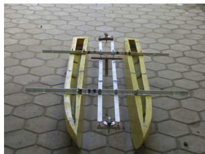
Fig. 6. Catamaran model without hydrofoil
