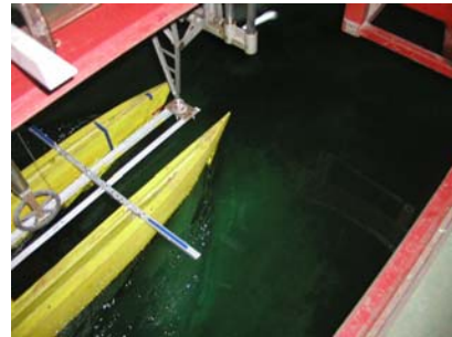
Fig. 13. Flow pattern around the catamaran model with dihedral foil
