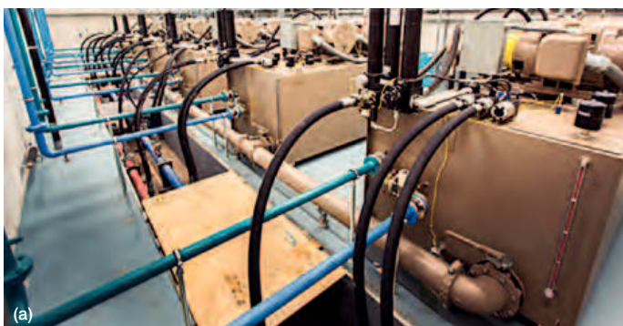
(a) hydraulic power units for wave generator (b) crane above flume to construct structures to be tested (c) blue wave paddle
