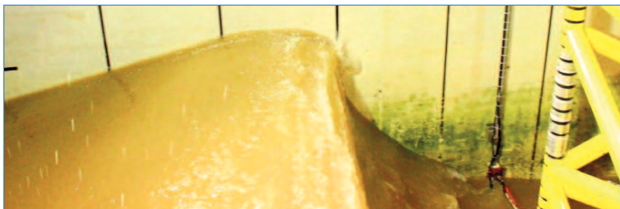
Figure 2 - Focussed wave generated using self-correcting method in shallow water in front of a truss structure (courtesy of LUH)
