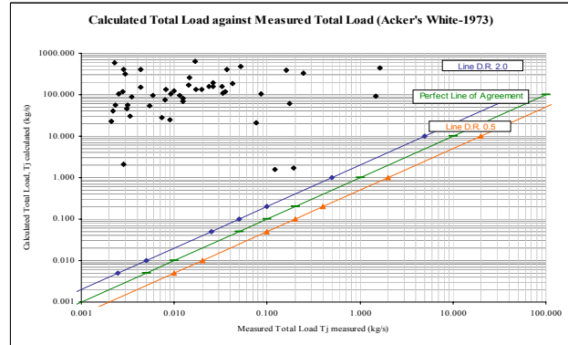
Figure 9: Comparison of measured and predicted sediment discharges using Ackers & White (1973) Equation
