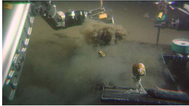
Figure 3 The sampling of submarine sediment with the use of manipulators of Hyper Dolphin. The scene is not clearly seen because of suspension of sediment.
