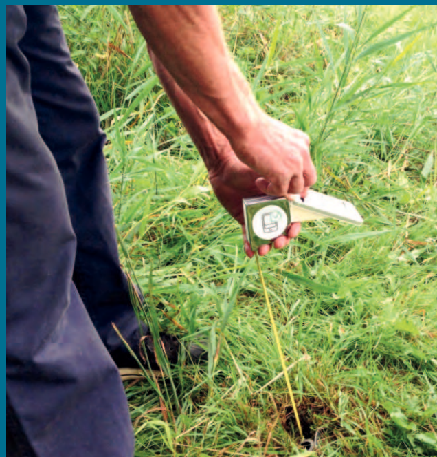
Figure 3. Mobile Tracker measuring a ground water level
