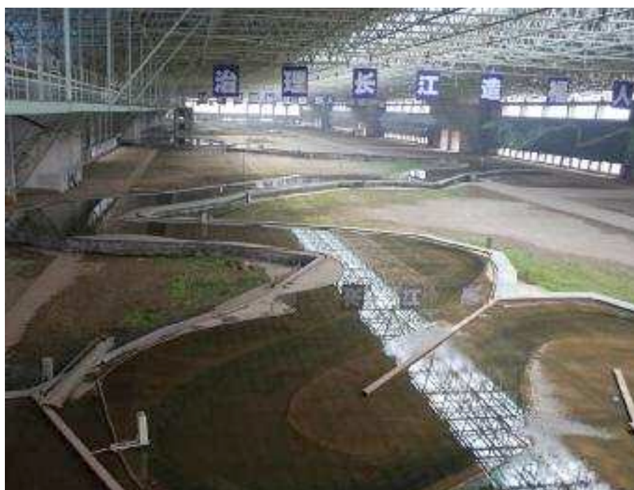
Figure 4. Immovable bed model tests
