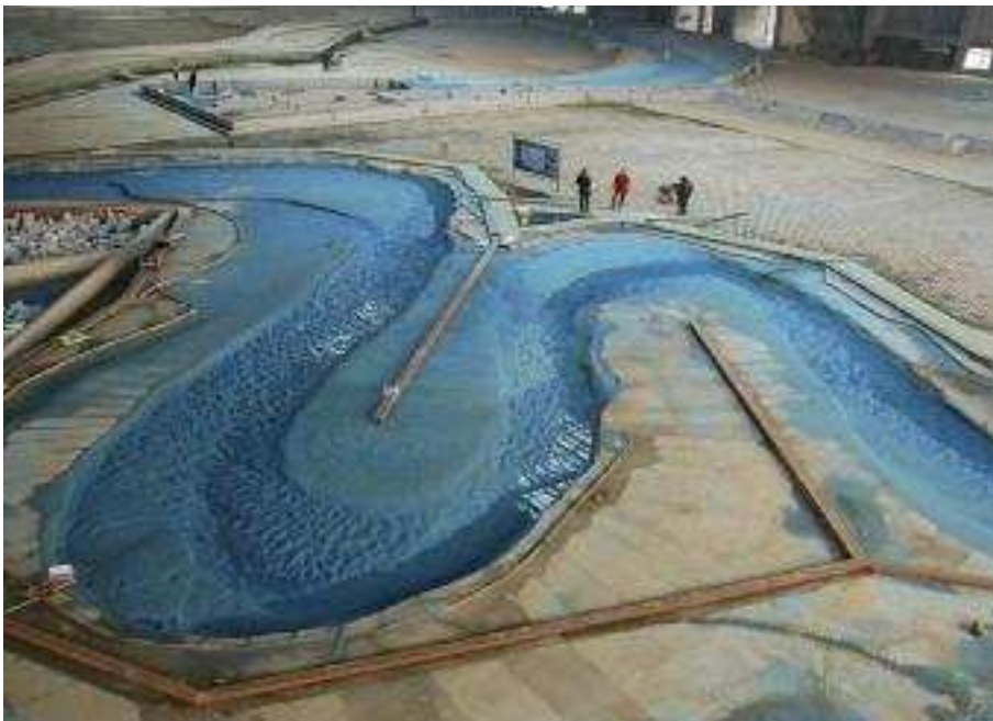
Figure 5. Movable bed model tests (with blue)
