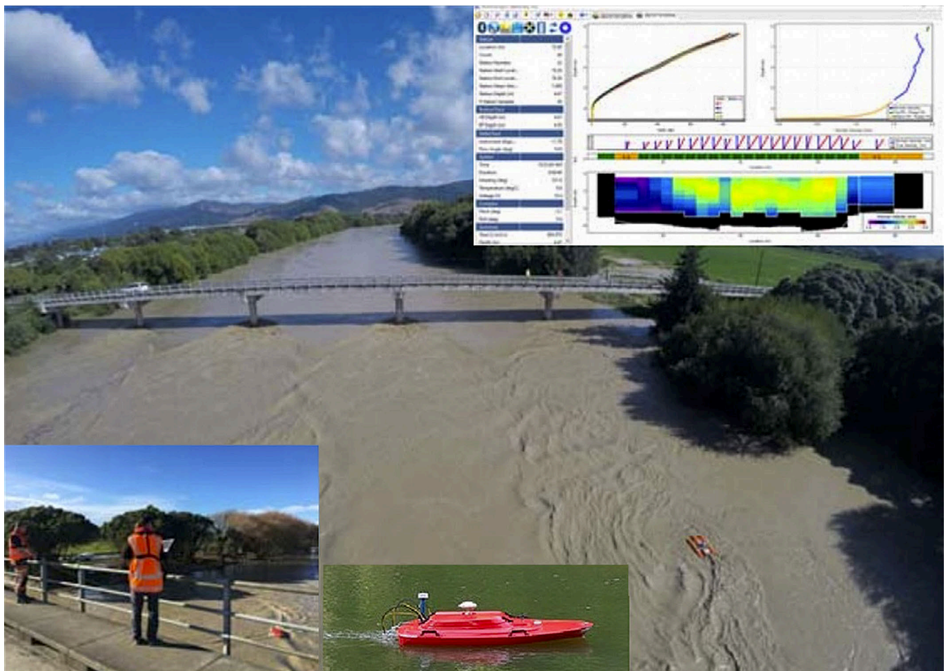
Figure 4 | ADCP gauging a major flood using a remote-controlled boat.
