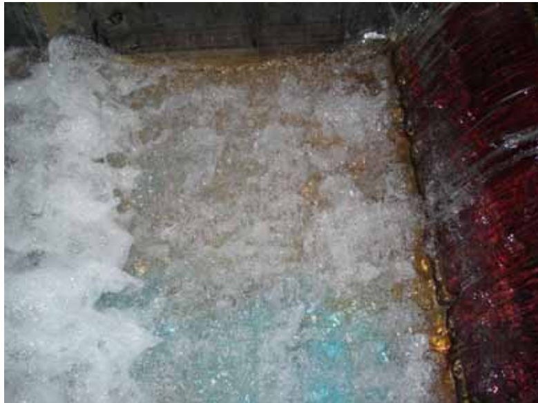
Figure 5: Flow pattern for condition of some tailwater existence at the downstream of weir
