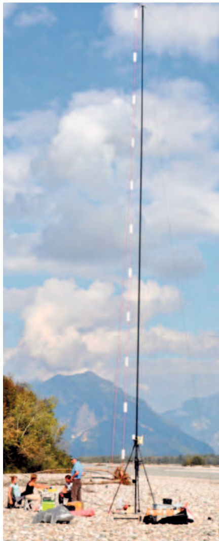
Fig. 3 Measurements of wind profiles over the floodplain of the Tagliamento.
