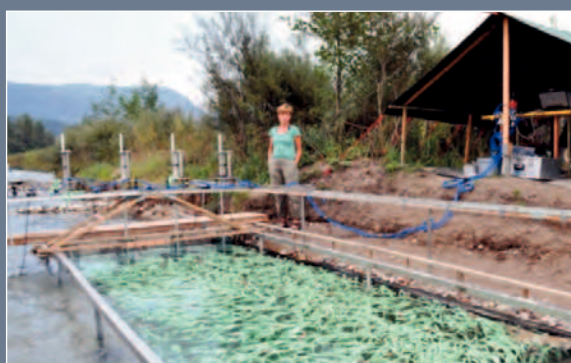
Fig. 2 Experiments in vegetated groyne fields with rigid emergent vegetation (left), and flexible submerged models of aquatic plants (right).
